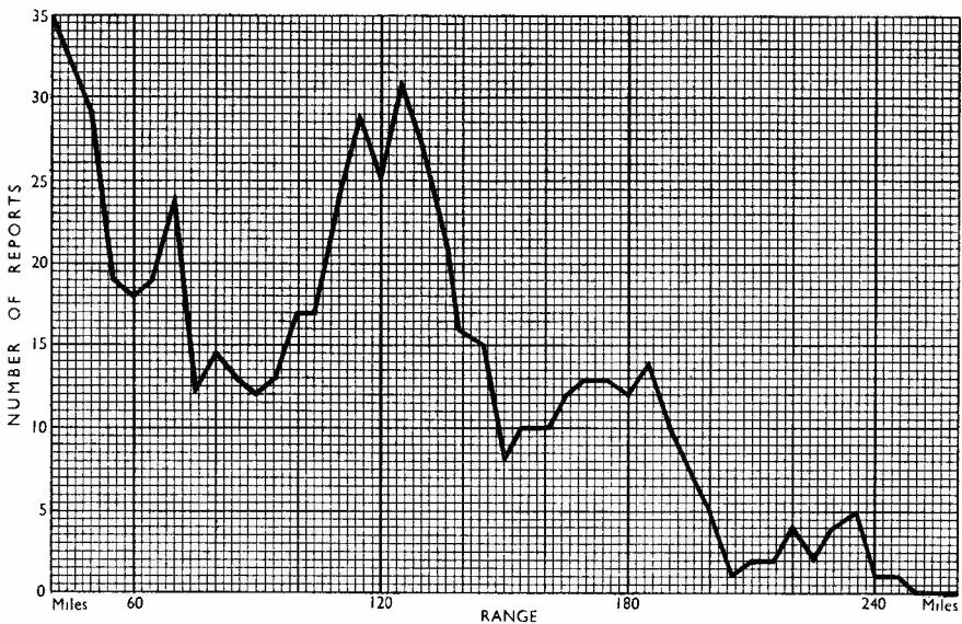
Fig. 3. The curve obtained by totalling all reports for the period May-November, 1946, as given in "Five Metres" in those issues. The 60-mile periodicity is very clearly shown. The author's contention is that this evidence points very strongly to the existence of a low-level ionised layer capable of returning 58 mc waves.
