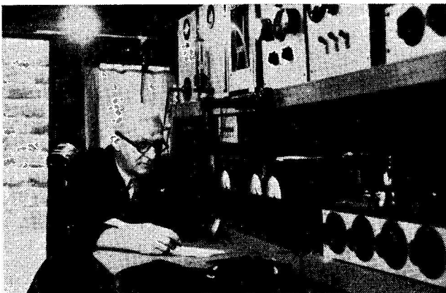
G6NP, Heckmondwike, Yorks. One of the trio featured in “100 Years of Amateur Radio” in the September issue. The transmitter equipment is on the upper shelf and on the operating bench is an RME-69 with DB-20 pre-selector.
