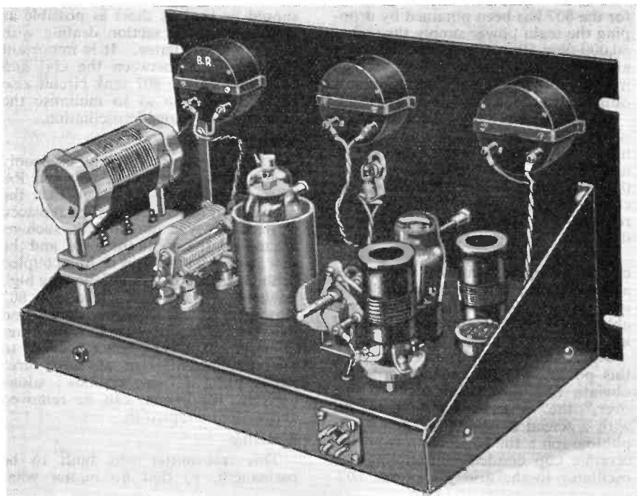
Half-rear view of the chassis. The 807 PA is in a screening can, with output tank coil and condenser to its left. The panel and chassis are of steel and obtainable in standard sizes for assemblies of this kind.
